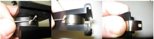
4. Bring end of spring between plastic piece and metal part of pusher assembly and push hole over tab on pusher. Be sure that end of spring is firmly seated and hooked on undercut of tab on pusher.
