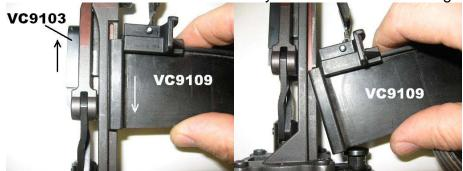
Assembly is in reverse order. Note that **VH0461** acts as a stop for **VC9103 slide**, you must push the slide and jaws forward to reinstall **VH0461**. If the slide is **not pushed forward** during screw installation, **breakage** of the slide **will occur**.
