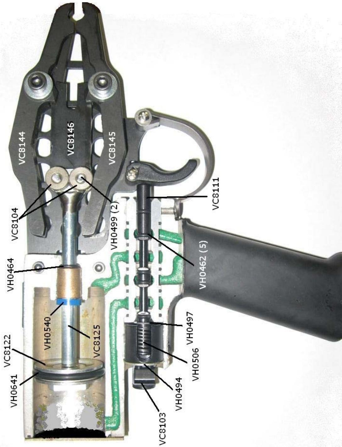
**Internal Components of VA0375 C-Ring Tool**
