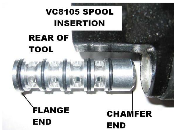
3. Use light amount of grease **VH0214** on valve rod **VC8111** and o-rings **VH0462**.
