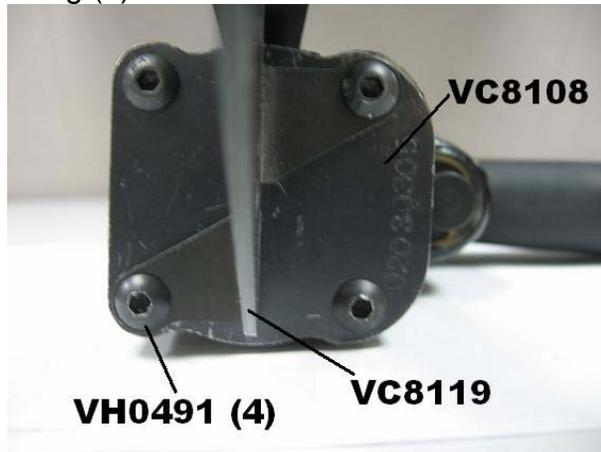
7. Remove end plate **VC8108** and o-ring **VH0496**.
