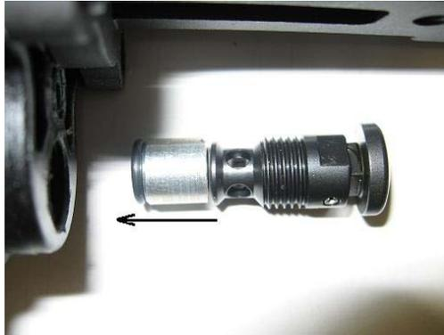
4. Coat end of **trigger assembly VC9116** lightly with grease to prevent o-ring from twisting, and install trigger into housing. **(DO NOT OVER TIGHTEN.)**
