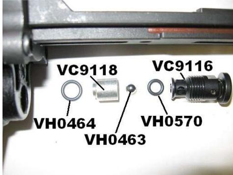
3. Assembly is in reverse order. Assemble **o-ring VH0464**, **valve seat VC9118**, **ball VH0463** and **o-ring VH0570** and insert into bore of housing, apply grease to both ends.
