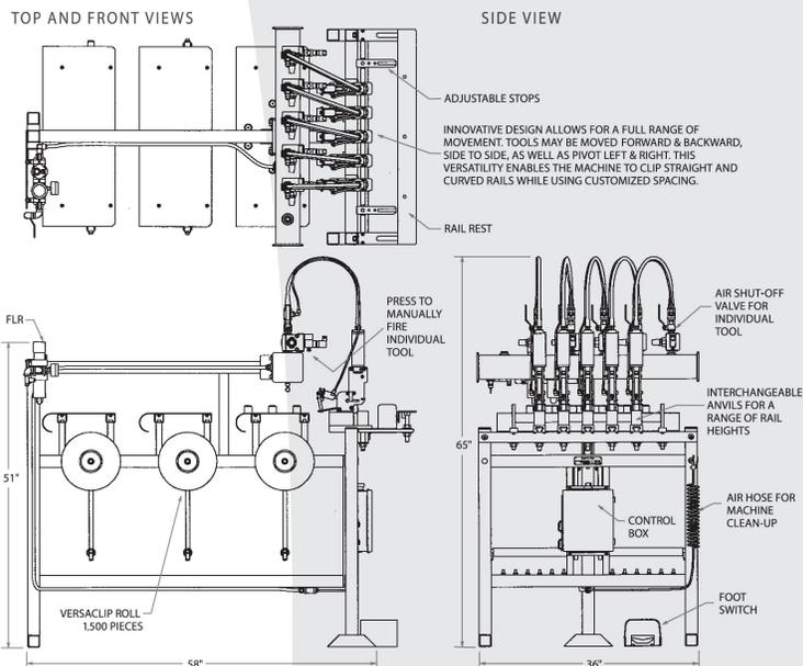
VersaClips™ covered by Patent No. 5,833,064. VersaClipper™ is covered by one or more of the following patents: 5,303,821; 5,833,064; 6,055,716.
