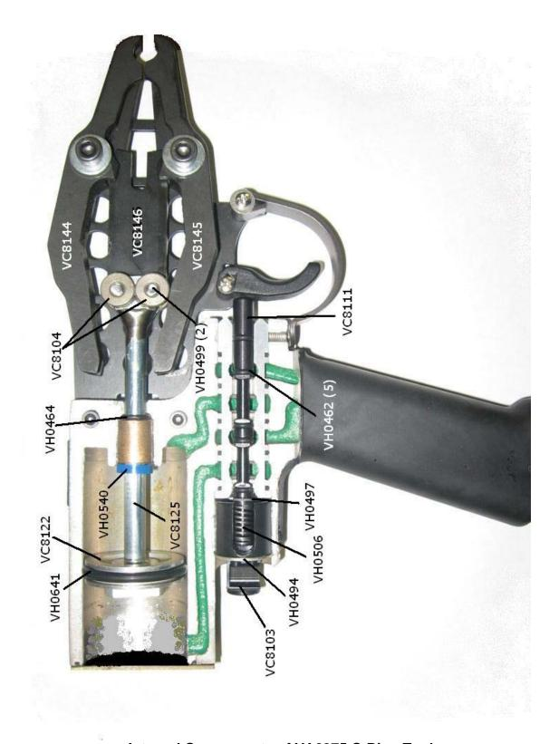
Internal Components of VA0375 C-Ring Tool
